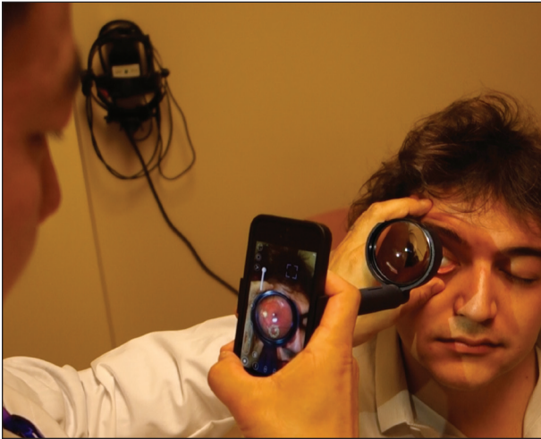
Figure 2. The EyeGo posterior segment adapter in action, showing the retina of coinventor Alexandre Jais.
