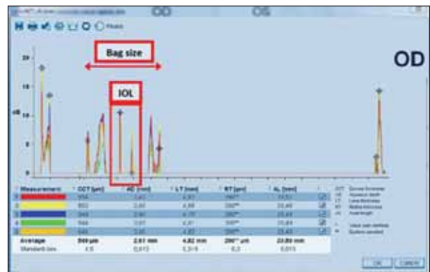
Figure 6. Lenstar LS900 scan of an eye before surgery allows the measurement of corneal thickness (CCT), anterior chamber depth (AD), lens thickness (LT), and axial length (AL) using PCI. The postoperative scan of the eye documents the position of the IOL, which has been implanted in the bag.
