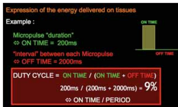
Figure 6. Micropulse duty cycle is an expression of the energy delivered to retinal tissues.
