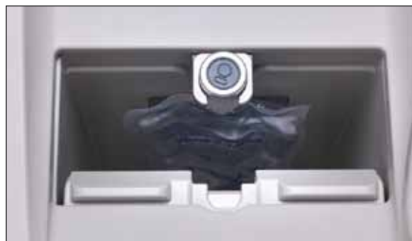
Figure 1. Active Fluidics Technology tightly controls inflow fluid pressure by placing the BSS bag (Alcon Laboratories, Inc.) between two compression plates that dynamically respond to the events of surgery.
