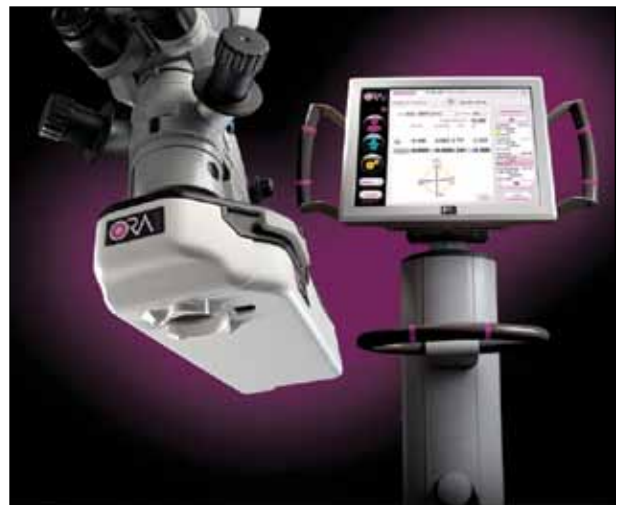
Figure 1. The ORA System is used for intraoperative wavefront analysis.
