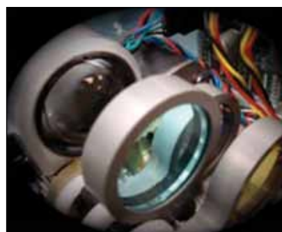
Figure 3. Three surgeon-controlled filters provide optimized visualization and additional safety and differentiated viewing.
