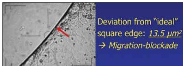
Figure 3. The deviation from the ideal square edge for migration blockade is 13.5 \mu\text{m}^2 .
