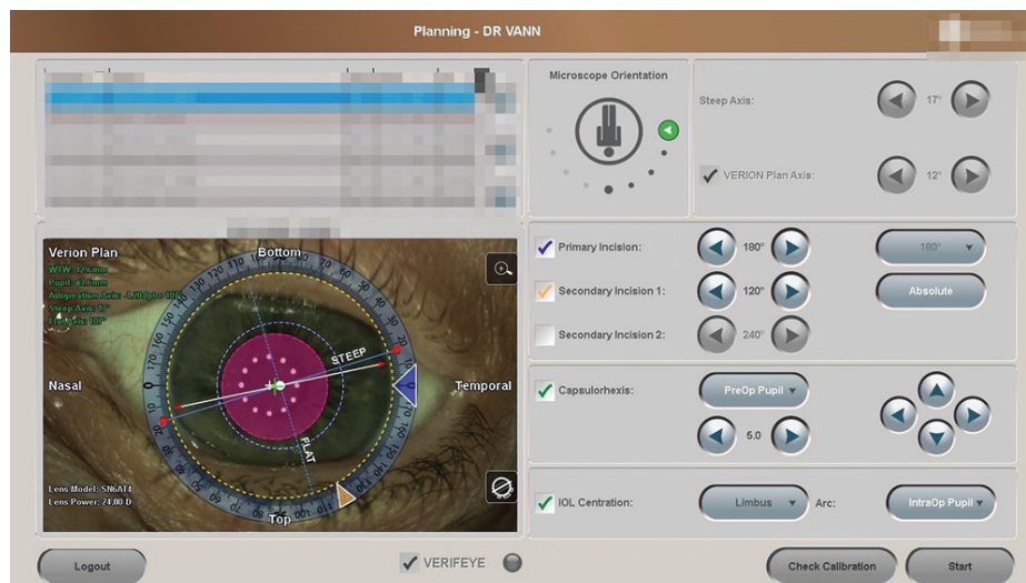
Figure 2. The Verion intraoperative planning screen allows you to determine the microscope relation to the patient for real time tracking and overlay incision orientations and capsulorhexis guides. The IOL centration and orientation can be adjusted according to the preoperative limbus, preoperative pupil or visual axis.
