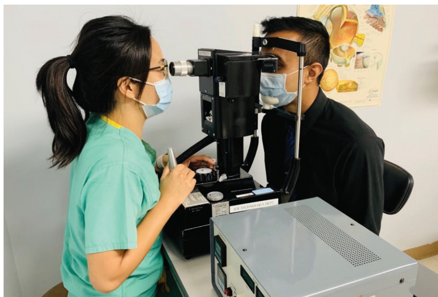
Figure 1. The Belmonte aesthesiometer uses a noncontact air jet to provide mechanical, thermal, and chemical stimuli.
