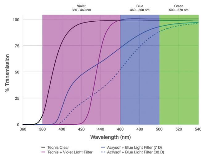
Figure. Transmission spectra of various IOLs, including those with violet-light- and blue-light-filtering chromophores. Note the steep IOL power-independent cutoff of the violet-light filter versus the broad cutoff of the blue-light filter, which moderately reduces the transmission of important blue light while allowing the transmission of high-energy phototoxic violet light, especially in lower-diopter IOLs.
